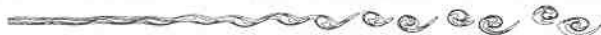
Fig. 13 Contours of constant vorticity of the simulated free shear layer perturbed by the most unstable mode and its subharmonic.
