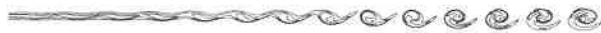
Fig. 11 Contours of constant vorticity of the simulated free shear layer perturbed by the most unstable mode at a magnitude of one hundredth.
