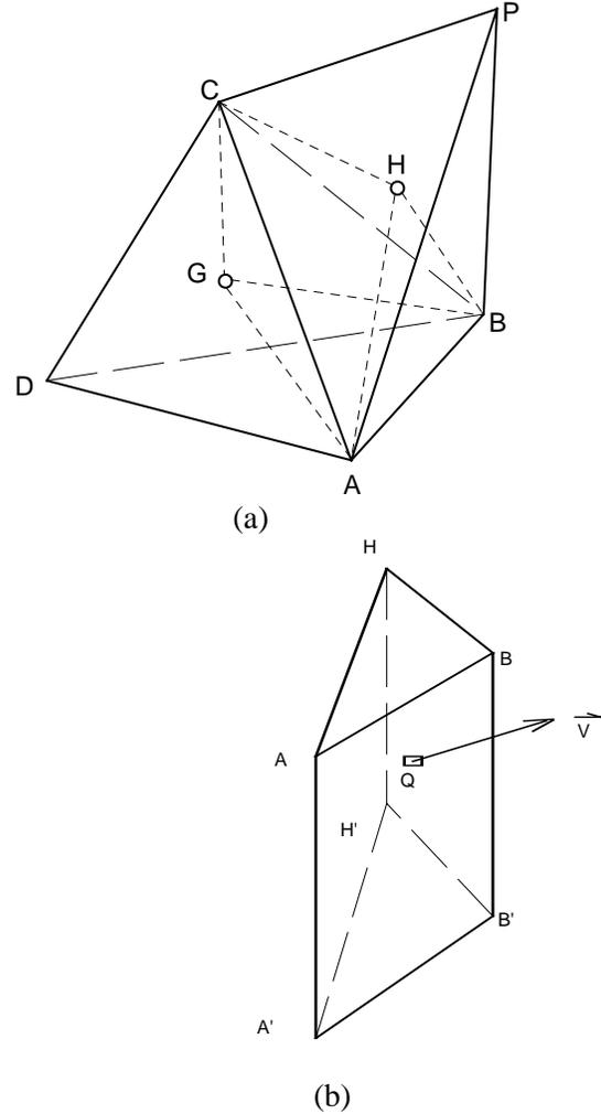
Fig. 2.1 (a) The definitions of the CE and SE; (b) The calculation of the viscous flux
