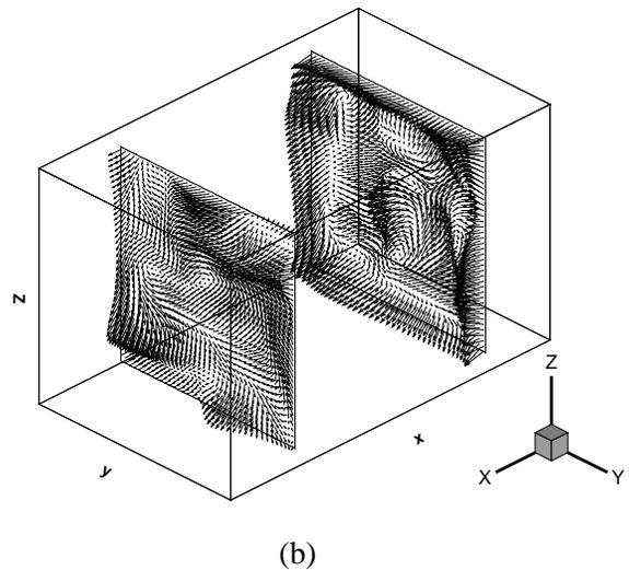
Fig. 3.1, (a) The schematic of the 3-D driven cavity flow; (b) Velocity vectors on two different  $x$ - $z$  planes; (c) Velocity vectors on the mid  $x$ - $y$  and  $y$ - $z$  planes; (d) and (e) Velocity vectors and pressure contours on the mid  $x$ - $z$  plane, respectively; (f) Velocity  $u$  distribution on the  $x=0.5$  and  $y=0.5$  central line.
